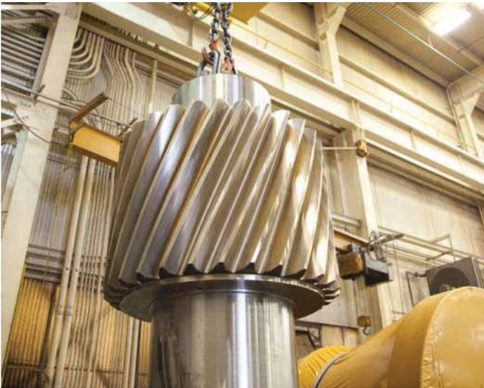
New pinions can also be designed and manufactured using this process, providing you with savings on material and heat treating versus an integral shaft. It also allows us to vary the material of the shaft and the shell for different hardness combinations that will best meet your needs. Whether carburized or through hardened, the shell on shaft combination will be an upgrade to your present pinions.
