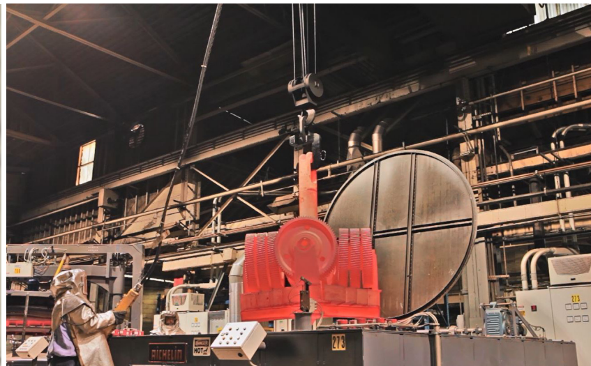
Carburizing and hardening with surface combustion pit furnaces for large gear treatment.
