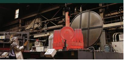
**Carburizing and Hardening** with surface combustion pit furnaces for Large Gear Treatment.
