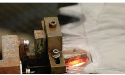
**Induction Hardening** for stronger gears that stand up to high stress usage, increasing Gear Life and Productivity.
